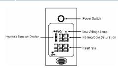
The length of the bargraph indicates the intensity of the pulse
